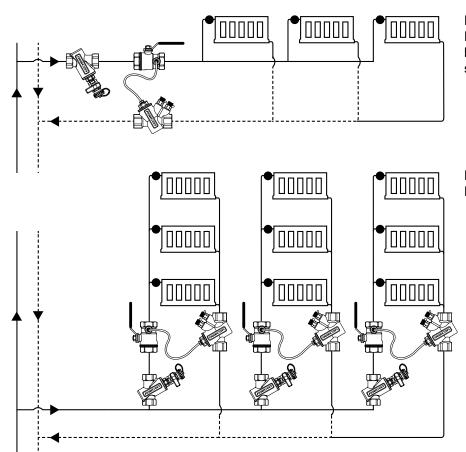
FlowCon SDP mounted with FlowCon Partner Ball on the branch in a 2-pipe heating system.
