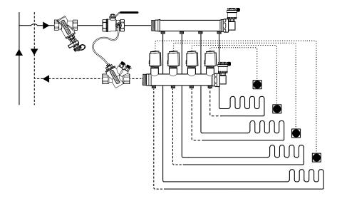
FlowCon SDP mounted with FlowCon Partner Ball on a manifold in an underfloor heating system.
