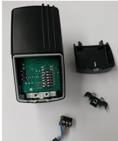
Pull the cable bayonet connection off the pins
