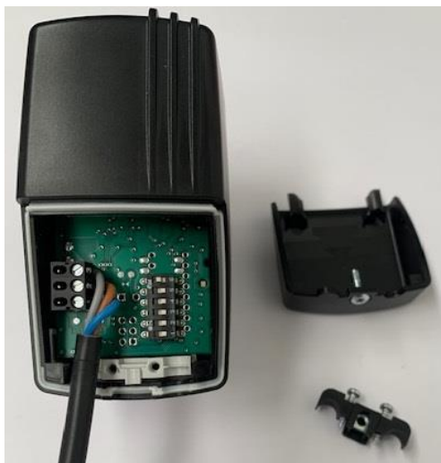
Remove the cable retaining clip using a Torx T7 driver
