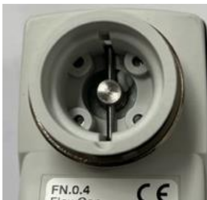
The S.S drive pin should be fully up
