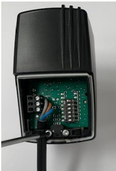
Remove the cable retaining clip using a Torx T7 driver
