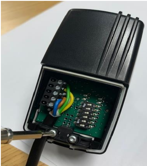
Remove the cable retaining clip using a Torx T7 driver
