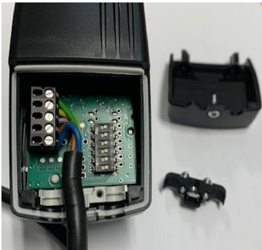
Remove the cable retaining clip using a Torx T7 driver
