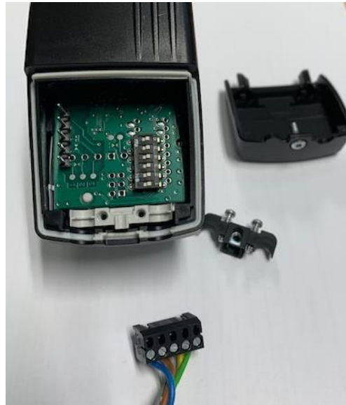
Pull the cable bayonet connection off the pins
