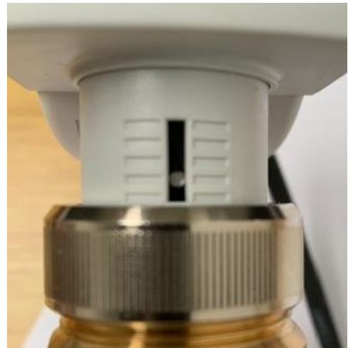
The closed position for the Green.2
