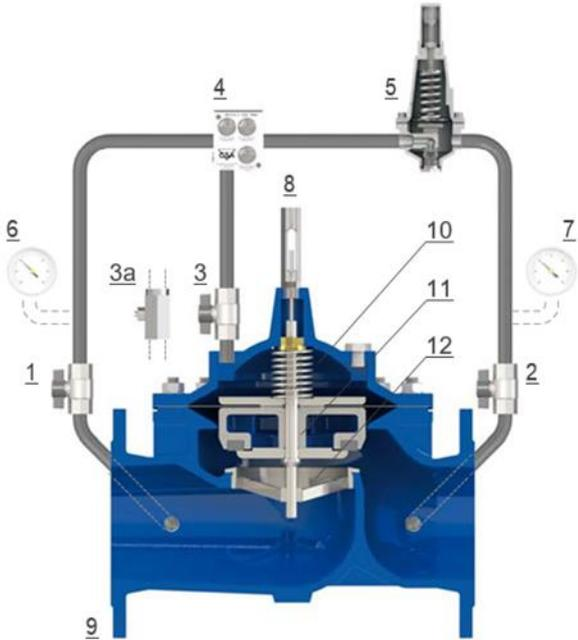
The DNS models XLC 310/410 are automatic control valves operated by a 2-ways pilot (5) with pre-set set and adjustable value.
