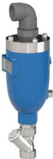
The Air Valve DNS-3F-AS-HR ensures proper system operation allowing the release of air pockets during working conditions, the intake of large volumes of air during draining operations and pipeline bursts and air discharge with controlled speed, to prevent water hammer.
