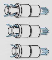
Within the operating pressure differential range, the effective open orifice area of the insert is automatically adjusted to the point where the specified flow rate will be delivered (as the pressure differential increases, the open area closes and as it decreases, the area opens).
